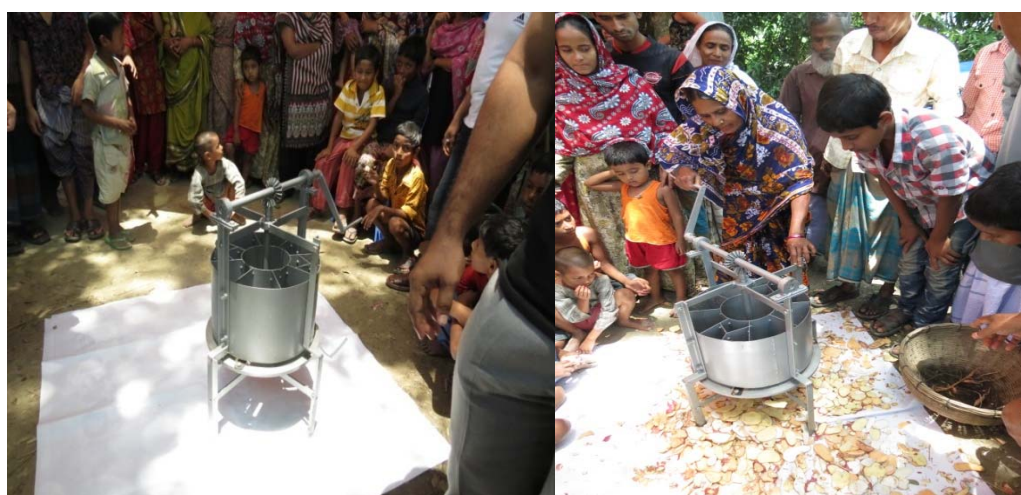
Pedal operated farmer-friendly cost effective Sweet potato Chipping machine
